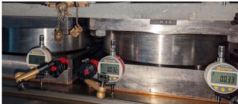
Measurement on outer ring (VLT)
