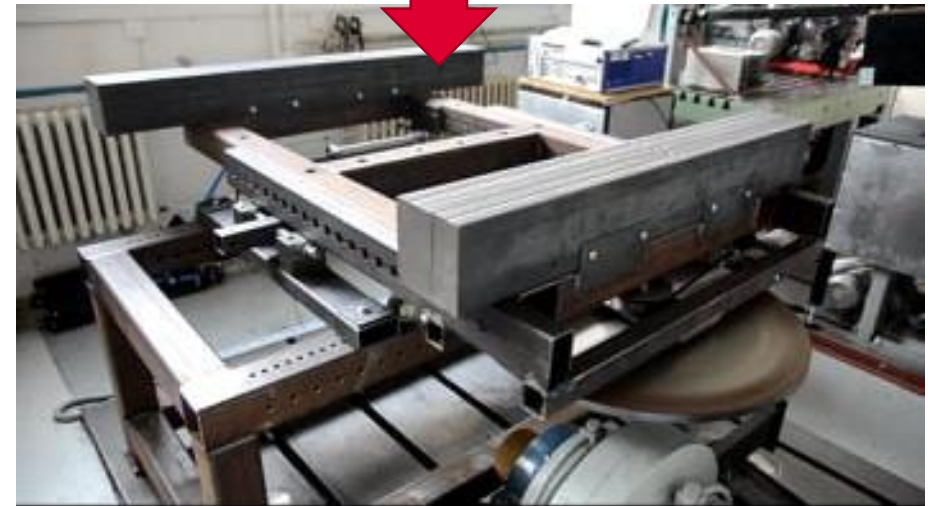
Verification of the function of the MR damper on the model of the rolling stock bogie
